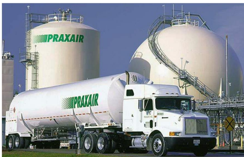
Figura 35 – Cryogenic-trailer para H 2 (Praxair, 2014)
